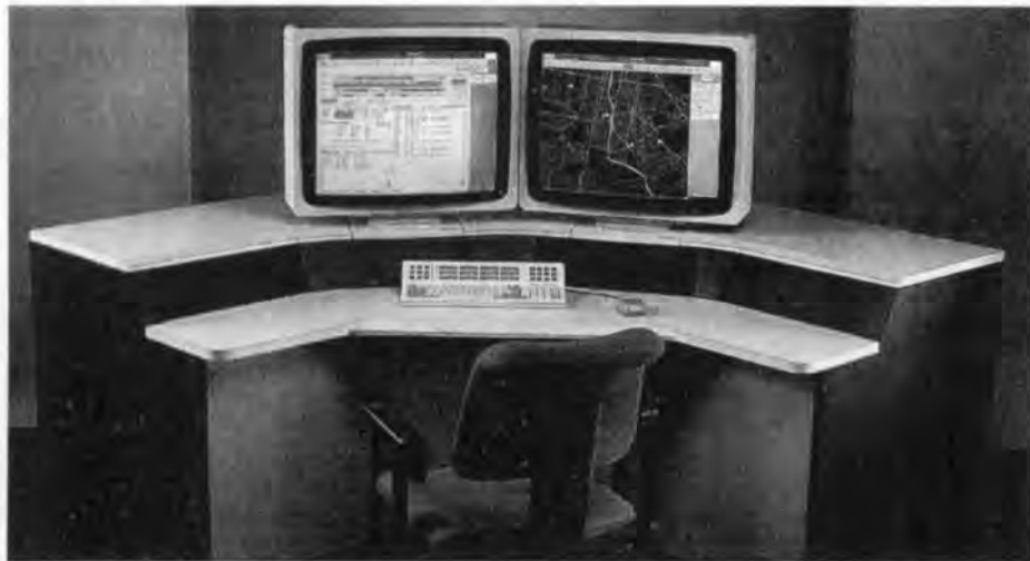
The Intergraph dispatcher workstations consists of one monitor for dispatch queuing and one for a map display capable of showing vital information about resources available at any particular time. The system is also capable of tracking duplicate calls to the same incident.
