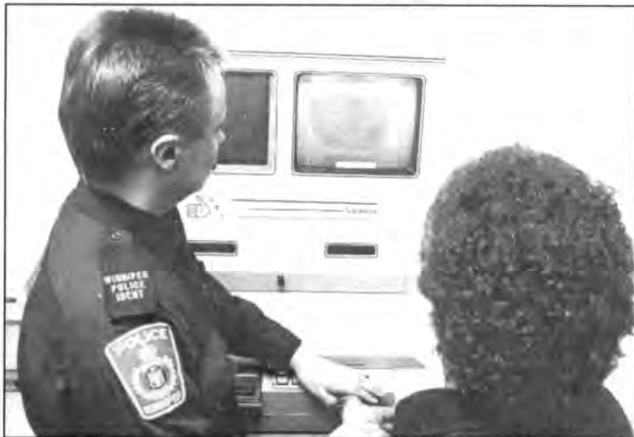
The Winnipeg Police Department's TenPrinter system scans subjects' fingerprints and then sends them directly to an automated fingerprint identification system (AFIS), allowing for instant identifications. Ident Technician Daryl Francis is shown demonstrating the new instrument.
