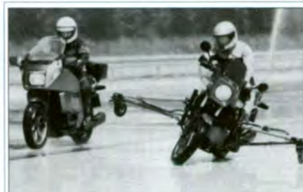
The outrigger-equipped motorcycle, without ABS, has locked up the wheels and lost stability during hard braking on wet pavement (right). The ABS-equipped bike remains upright and controllable under the same conditions (left).
