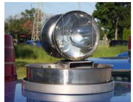
A snapshot of the motor-driven version of the red “bubble” overhead light, and shown at left on a 1970s-era Plymouth Fury.
