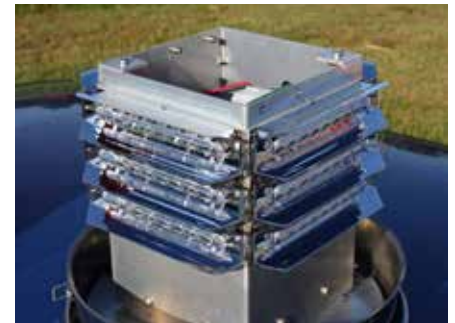
The new LED overhead light, shown on the MSP’s Dodge Charger at left, produces an intense, wide-angle red light in all directions that only requires three amps to operate. Each kit uses 12 light heads, nine LED bulbs per head, for a total of 108 lights in each car.
