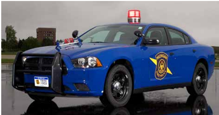
The new LED overhead light, shown on the MSP’s Dodge Charger at left, produces an intense, wide-angle red light in all directions that only requires three amps to operate. Each kit uses 12 light heads, nine LED bulbs per head, for a total of 108 lights in each car.
