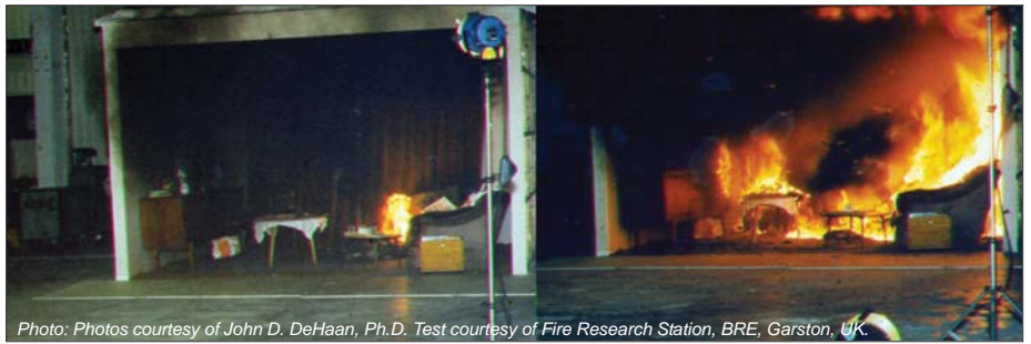
Figure 3: Stages in the development of a fire. These three photos show a newspaper fire in a plastic bin (upper left) six minutes after ignition, at rollover (upper right) nine minutes after ignition and 10.75 minutes after flashover (lower left).
