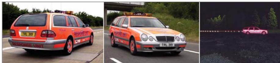
Figure 3. Retro reflective edge markings and uniform colour intended to enhance vehicle conspicuity (Source: Fay and Sferco, 2002)
