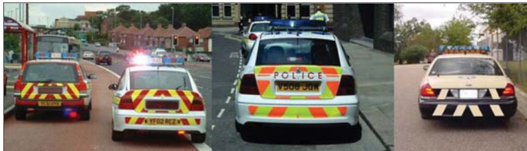
Figure 1. Rear-end Chevron patterns for police vehicles in three colour schemes. (Source: Wells, 2002)
